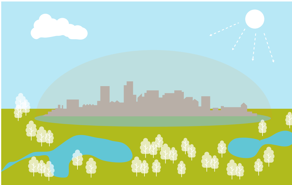
› Figure 3 - The paved surfaces create a dome, which traps the heat origin from sun radiation and human activities. The cooler air at higher levels of the atmosphere traps heat within the cities.
